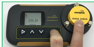
While the reading is visible, press ^ or v , the display will then show 0.0 , press ⓪ to display Grain Cell temperature.
